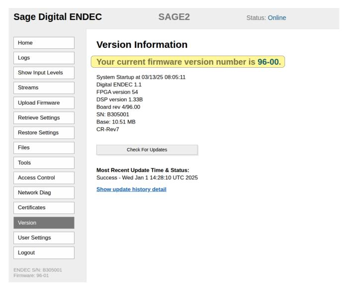
Figure 1: Version page, showing that firmware version 96 update was previously installed.
